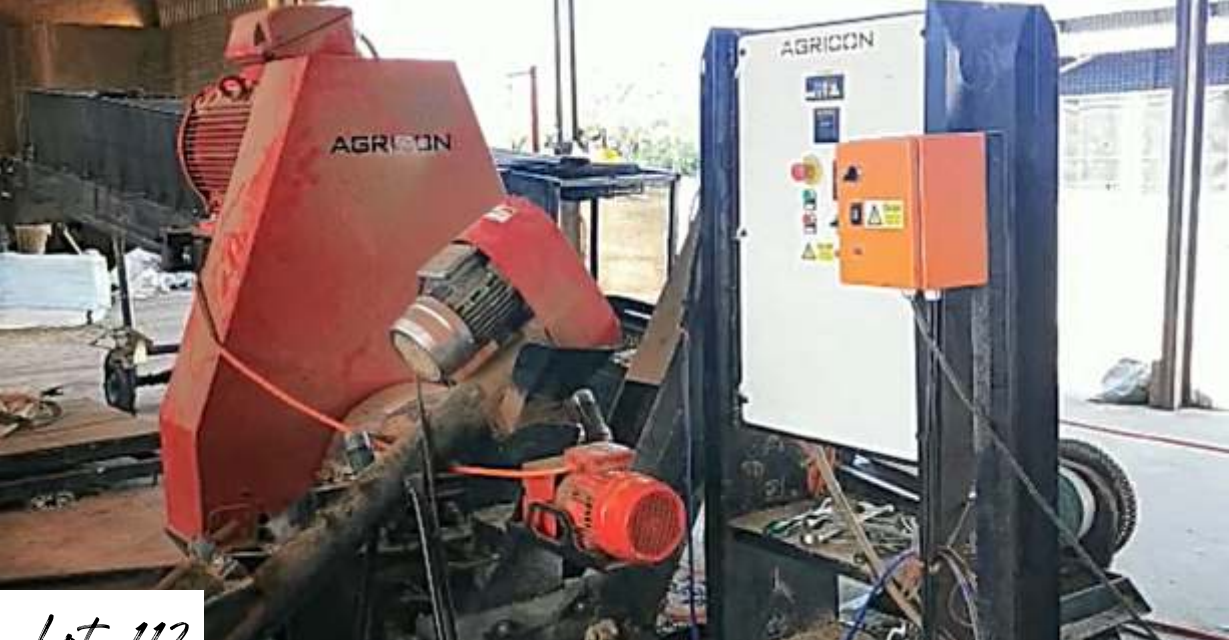
Agrocon 150 Pelletizing Plant (1,5 ton p/h), 45 kw (100 amps), Feed Auger with Variable Speed Drive to feed directly into Agrocon Machine Bucket Elevator 1.6m for 2 x 50kg bag filling with double attachments & separate handle
